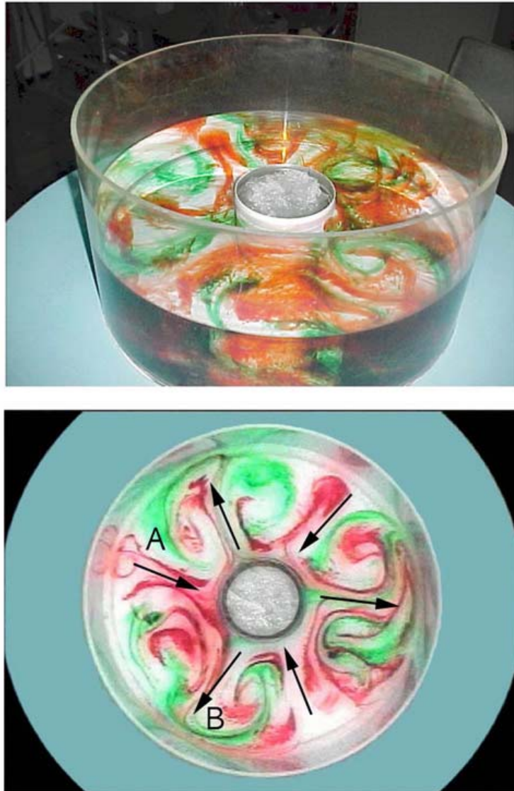
Figure 8.7: (Top) Baroclinic eddies in the 'eddy' regime viewed from the side. (Bottom) View from above. Eddies draw fluid from the periphery in toward the centre at point A and vice-versa at point B. The eddies are created by the instability of the thermal wind induced by the radial temperature gradient due to the presence of the ice bucket at the centre of the tank. The diameter of the ice bucket is 15 cm.
