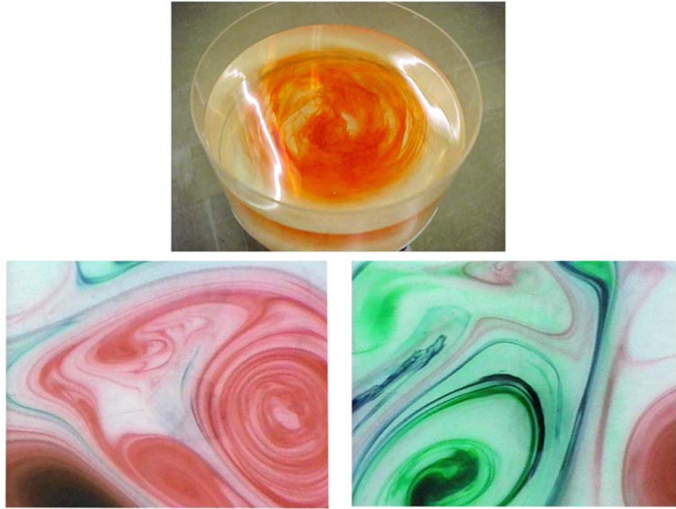
Figure 6: Taylor columns revealed by food coloring in the rotating tank. The water is allowed to come into solid body rotation and then gently stirred by hand. Dyes are used to visualize the flow. At the top we show the rotating cylinder of water with curtains of dye falling down from the surface. Below we show the beautiful patterns of dyes of different colors being stirred around one another by the rotationally constrained motion.
